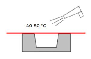
3) When temperature is confirmed, press the film into the deepest part of the corrugation/recess, using your finger. Start always from the deepest part of the corrugation where the maximum stretch is required for the material. To facilitate sliding of the finger, wear Mactac Glove and wet your finger with soapy water. Ensure 100% contact between the surface and the vinyl.
