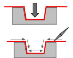
6) Once all the film is in contact with the profile, press firmly again with the squeegee. Check the complete application and prick any air bubbles using the appropriate tool.
