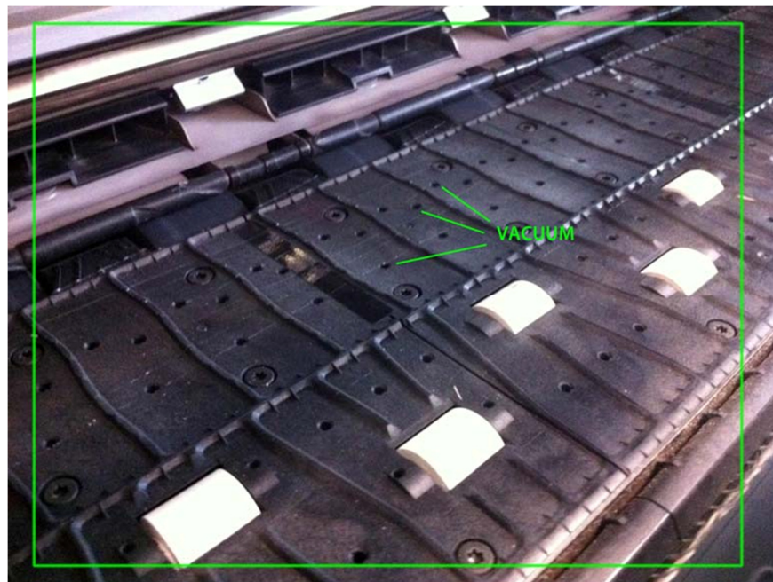
5 - A closer look to the print platen of a HP 25500 latex printer
