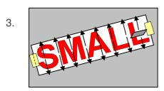
Position the lettering or the logo once again on the spot marked by the piece of positioning tape.
